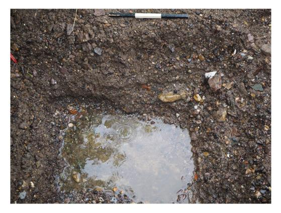
Figure 4 – This photo was taken approximately 30 seconds after the one above (Fig 3) and illustrates the rate that water was ingressing into the trench.
